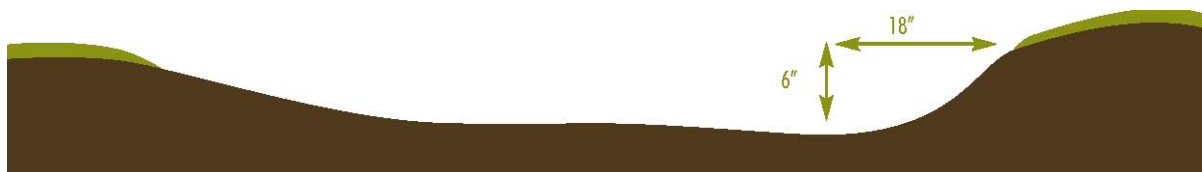
Figure 6. Sloping the Sides of a Rain Garden
